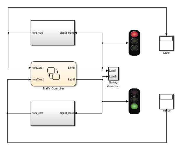
Inside the Traffic Controller chart, two parallel subcharts manage the logic controlling the traffic lights. The subcharts have an identical hierarchy consisting of three child states: Red, Yellow, and Green. The output data Light1 and Light2 correspond to the active child states in the subcharts. These signals:
