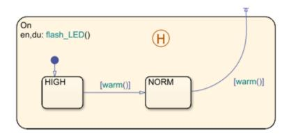
As a result, the timing of the status LED depends on the operating mode of the boiler. For example:
