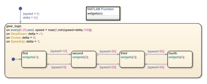
You can execute this chart as an object in MATLAB directly through the Command Window or by using a script. You can also program a MATLAB app that controls the state of the chart through a graphical user interface. For example, this user interface sends an input event to the chart when you click a button. In the chart, the MATLAB function widgets controls the values of the gauges and lamps on the interface.
