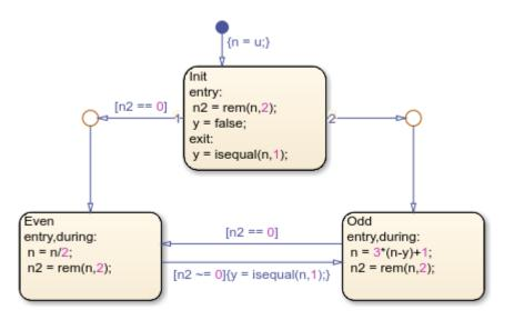
The chart consists of three states. At the start of simulation, the Init state initializes the chart data:
