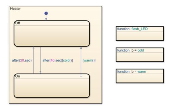
The labels on the transitions between the  ${\tt On}$  and  ${\tt Off}$  substates define the behavior of the bang-bang controller.
