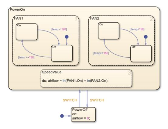
The controller operates two fans. The first fan turns on when the air temperature rises above 120 degrees. The second fan provides additional cooling when the air temperature rises above 150 degrees. The chart models these fans as parallel states FAN1 and FAN2, both of which are active when the controller is turned on. Except for their operating thresholds, the fans have an identical configuration of states and transitions that reflects the two modes of fan operation (On and Off).
