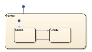
The contents of a parent state behave like a smaller chart. When a parent state becomes active, one of its child states also becomes active. When the parent state becomes inactive, all of its child states become inactive.
