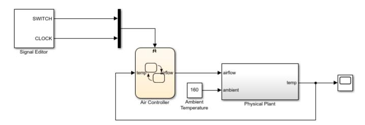
Based on the air temperature temp, the Air Controller chart turns on the fans and passes the value of airflow to the Physical Plant subsystem. This output value determines the amount of cooling activity, as indicated by this table.
